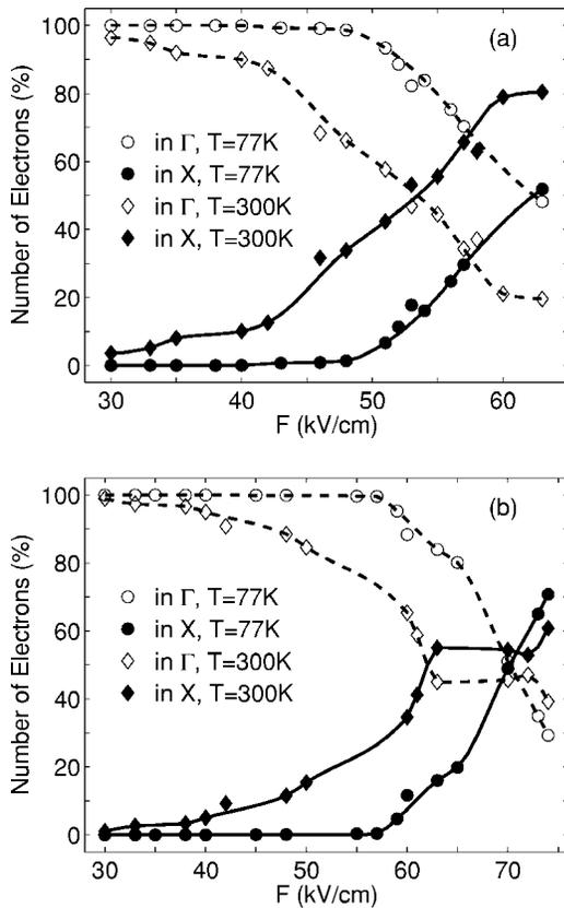
FIG. 3. Percentage of electrons in  $\Gamma$  and  $X$  valleys vs applied field for the 33% QCL (a) and the 45% QCL (b) at 77 and 300 K.
