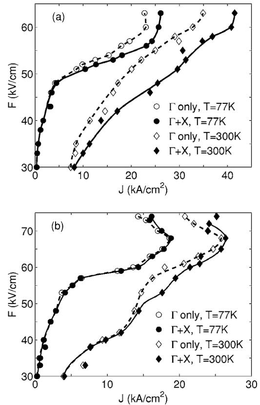
FIG. 2. Electric field vs current density characteristics for the 33% QCL (a) and the 45% QCL (b) at 77 and 300 K, with and without the X-valley transport included.
