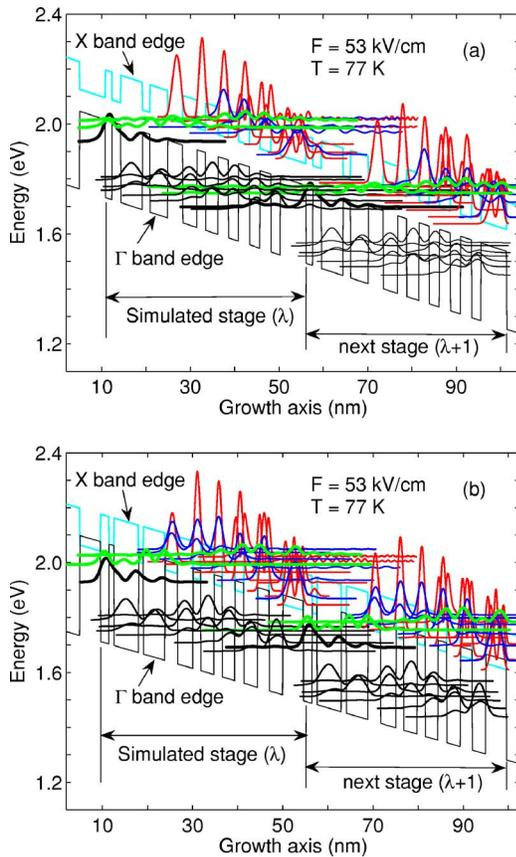
FIG. 1. (Color online) Energy levels and wave function moduli squared in two adjacent stages for the 33% QCL (a) and the 45% QCL (b). In each stage, the bold black line denotes the upper lasing level, while the thin black lines and two bold green lines represent the localized  $\Gamma_1$  states and continuumlike  $\Gamma_c$  states, respectively. X1 states (red lines) and X2 states (blue lines) in two adjacent stages are also shown.
