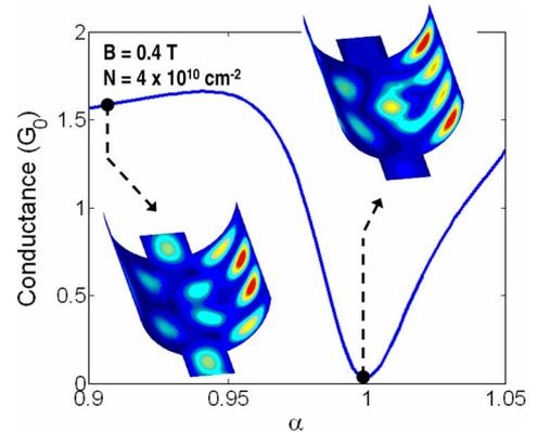
Fig. 4. Conductance variation with curvature at a low magnetic field ( $B = 0.4 \text{ T}$ ). Insets: colorized plots of the magnitude squared of the wavefunction at the Fermi energy, for the specific values of  $\alpha$  shown. Patterns observed in the probability density are altered by changes in curvature, significantly affecting the conductance.
