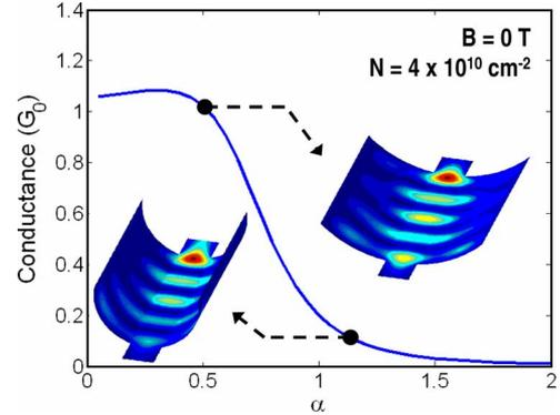
Fig. 3. Conductance variation with curvature at  $B = 0$ . At particular electron densities in the leads, the conductance is highly dependent on the curvature of the cavity even in the absence of a magnetic field. This phenomenon can only be attributed to the geometric potential. Insets: colorized plots of the magnitude squared of the wavefunction at the Fermi energy, for the specific values of  $\alpha$  shown.
