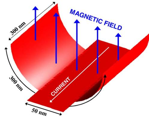
Fig. 1. A nonplanar resonant quantum cavity on a SiGe/Si heterostructure, formed by selective etching of the sacrificial layer under the cavity's wings. Strain from the lattice mismatch provides the force that causes the wings to bow. Curvature is measured in terms of  $\alpha = W/(\pi R)$ , where  $W$  is the width of the cavity and  $R$  is the radius of curvature.
