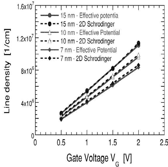
Fig. 3. Variation of the line charge density for a quantum wire that represents the channel region of the SOI device structure from Fig. 2. The wire width equals 7, 10 and 15 nm.
