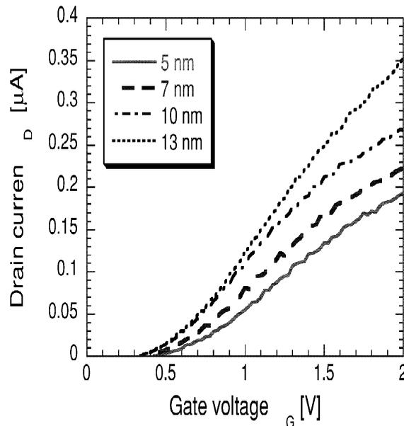
Fig. 4. Transfer characteristics of the SOI device with channel width equal to 5, 7, 10 and 13 nm. The drain voltage  $V_D$  equals 10 mV.
