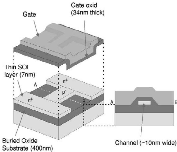
Fig. 2. Schematic description of the SOI device structure.
