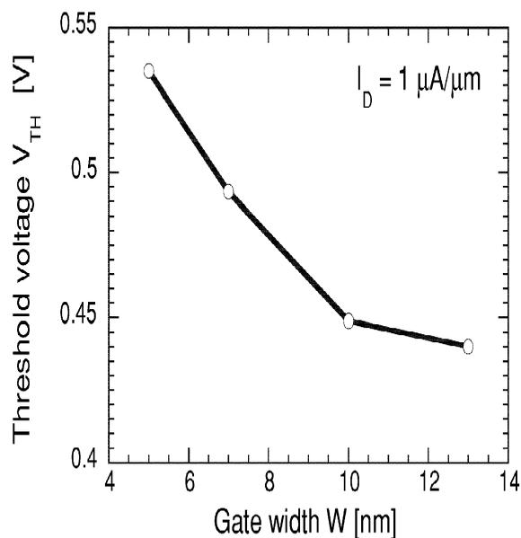
Fig. 5. Threshold voltage as a function of the gate width.
