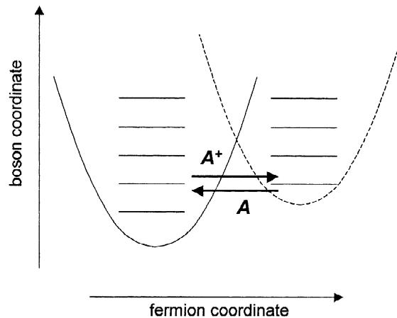
Fig. 1. The coordinates of the basic Hamiltonian and its partner. The left-hand potential (solid) represents that of  $H^{(-)}$  while the right-hand potential (dashed) represents that of  $H^{(+)}$ . The supercharge, and its conjugate, move laterally from one ladder of levels to the other.
