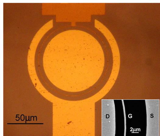
FIG. 1. (Color online) Optical microscope image of a circular MOSFET device ( $L_G=0.5 \mu\text{m}$ ). Inset: SEM image of the MOSFET gate region.
