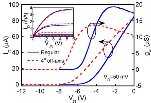
FIG. 2. (Color online) Comparison of the measured dc characteristics of MOSFETs with  $L_G=10\ \mu\text{m}$  and  $W_G=320\ \mu\text{m}$  fabricated on the regular (100) Si substrate (blue solid curves) and  $4^\circ$  off-axis Si substrate (red dashed curves). Linear transfer characteristics ( $V_D=50\ \text{mV}$ ) are presented in the main panel, while the inset features the  $I_D$ - $V_{DS}$  curves ( $V_G=-6$  to  $0\ \text{V}$ ; the step between successive curves is  $2\ \text{V}$ ).
