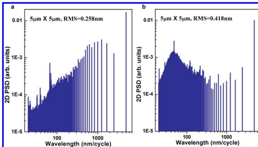
Figure 8. Two-dimensional power spectral density for two Si nanomembranes with different surface roughness: (a) rms = 0.258 nm; (b) rms = 0.418 nm. The scan area for both samples is  $5 \mu\text{m} \times 5 \mu\text{m}$ .
