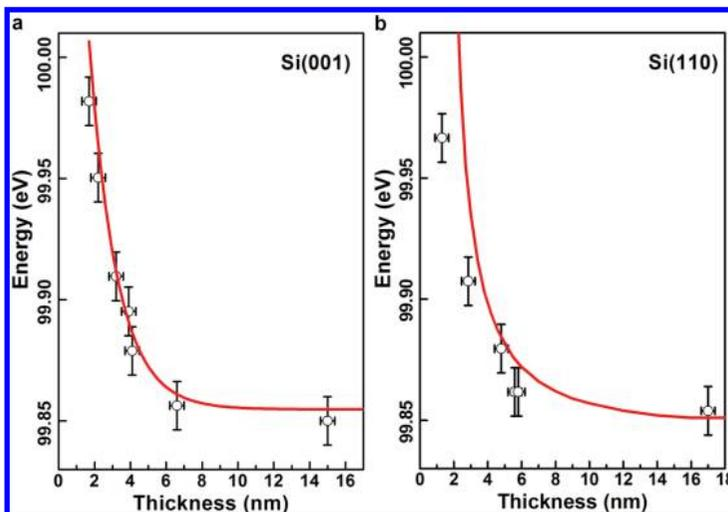
Figure 6. Quantum size effect: Shift of the weighted average  $\Delta$  valley energy as a function of the Si membrane thickness: (a) Si(001) and (b) Si(110). Symbols represent the measurements; solid lines represent the self-consistent calculation.
