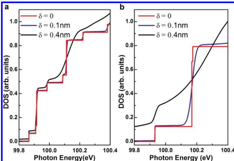
Figure 2. DOS for thin membranes and effect of roughness: (a) 5 nm thick membrane; (b) 2 nm thick membrane, both (001) orientation. The first large steps in the DOS correspond in both cases to the  $\Delta_4$  ground states, the first small steps correspond to  $\Delta_2$ . The energy scale is chosen to correspond to the transition from the  $2p_{3/2}$  core level of Si.
