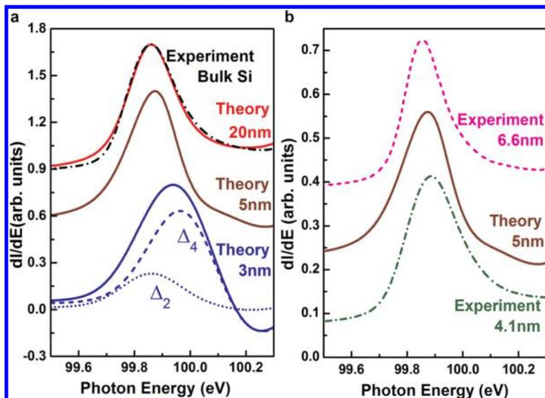
Figure 4. Calculated and measured derivative 2p-to- $\Delta$  absorption spectra for several membrane thicknesses. (a) Calculations at several thicknesses; 20 nm is the same as experimental bulk Si. The split  $\Delta_2$  and  $\Delta_4$  contributions to the peak for the 3 nm membrane are shown. The  $\Delta_2$  and  $\Delta_4$  peak separation increases with decreasing membrane thickness. (b) Comparison of the calculation for a 5 nm thick membrane with experiment for 4.1 and 6 nm thicknesses.
