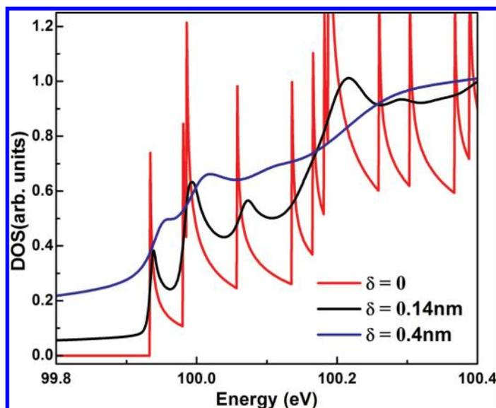
Figure 7. DOS of a 5 nm  $\times$  5 nm Si nanowire (red) and effect of two levels of surface roughness, 0.14 nm (black) and 0.4 nm (blue). The energy scale corresponds to the photon transition from the  $2p_{3/2}$  core level.
